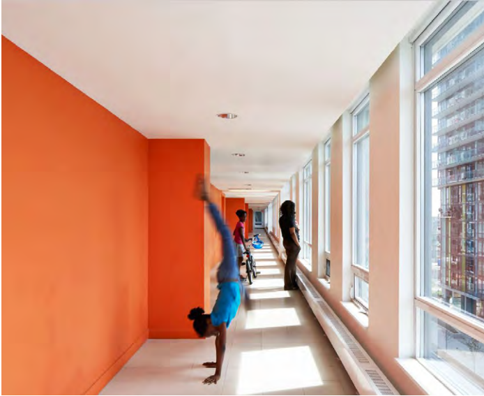
Hallways at 150 Dan Leckie Way in Toronto function as a social, play space. The building used the skip-stop typology which resulted in fewer corridors, providing them with the opportunity to become wider and naturally lit.
