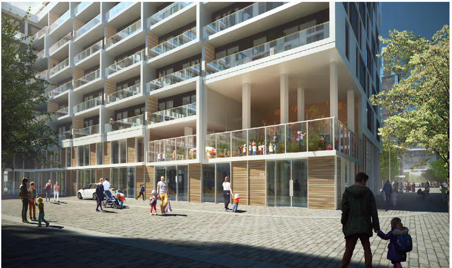
The Bayside development in Toronto shows how the child care's outdoor space was located on the 2nd level by taking a 'bite' out of the building. This alternative massing solution was a response to a constrained site and involved cooperation between the developer (Waterfront Toronto), City Planning and Children Services.
