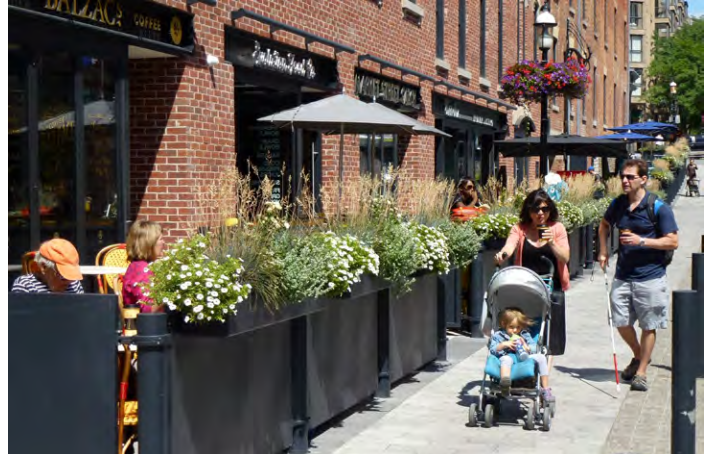
The reconfigured Market Street in Toronto introduced fine grain retail and patio seating. The shared street is a flexible design (which uses bollards instead of a curb) that better accommodates special events or pedestrians on market days.
